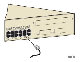
Figure 3-6 2E42-27/2E42-27R Twisted Pair Connection
